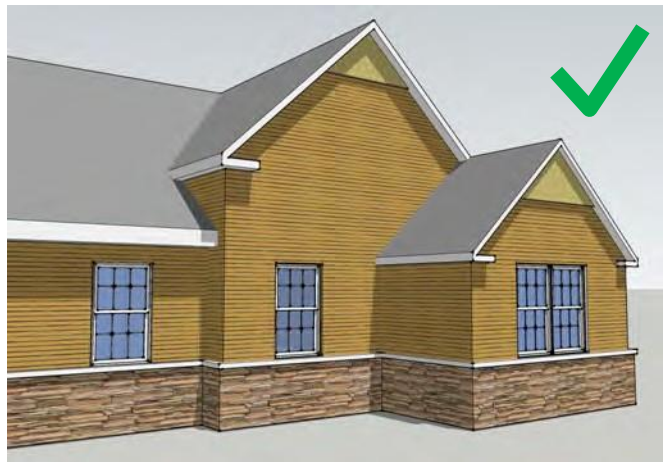
Figure 32. Attractive Building Massing. Simple shapes which are well defined and differentiated with changes in facade depth are encouraged.
