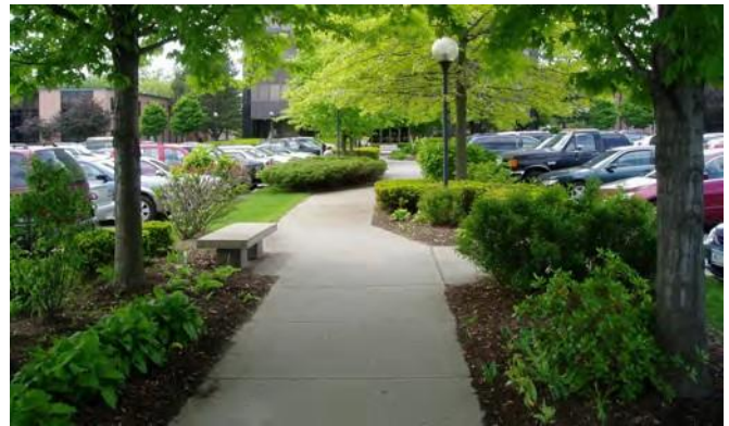
Figure 18. Dedicated pedestrian path. Dedicated pedestrian paths through a parking lot create a more attractive and safer shopping destination, giving people a safe route through the parking area.
