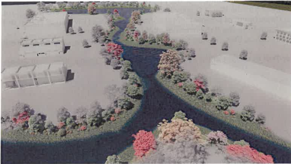
Figure 12 - Rendering of constructed stormwater treatment wetland-pond system. This green infrastructure practice of constructed wetland-shallow pond system that could be developed near an existing wetland or drainage corridor. Constructed wetlands are shallow marsh systems planted with emergent vegetation that are designed to treat stormwater runoff. They are extremely effective for pollutant removal and can mitigate flooding and reduce runoff volume. https://efc.ny.gov/green-stormwater-infrastructure#eligible-practices
